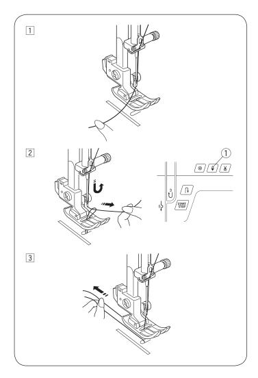
Drawing up the Bobbin Thread 1 Raise the presser foot. Hold the needle thread lightly with your left hand.
