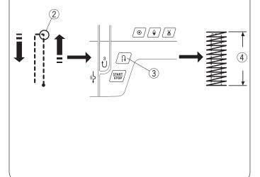
Tacking is used to reinforce pockets, crotches and belt carriers where extra strength is needed.
