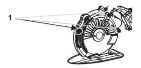
2. Align the positioning holes on the blade with the positioning holes on the back black cover.
