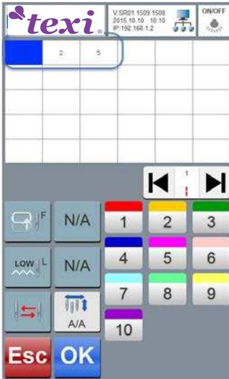
1. After the first colour has been embroidered, embroidery machine automatically stops working and the thread is cut, the needle bar automatically moves to the position which allows a second colour embroidery.
