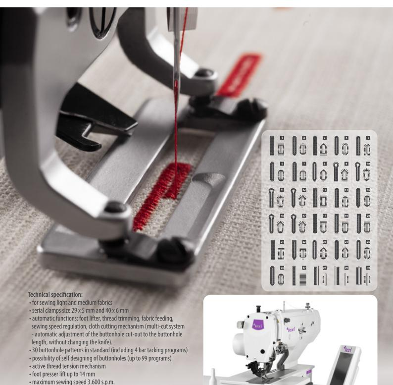
• integrated, energy-saving AC Servo motor and stepping motors
