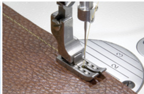
TEXI 5014 Roller foot for difficult fabrics
