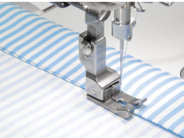
TEXI 5015 Foot with central tape guide 4.8 mm
