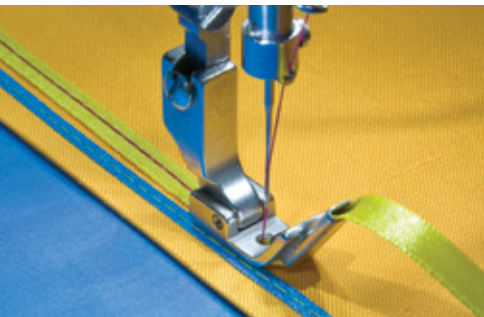
TEXI 5015 Foot with central tape guide 4.8 mm
