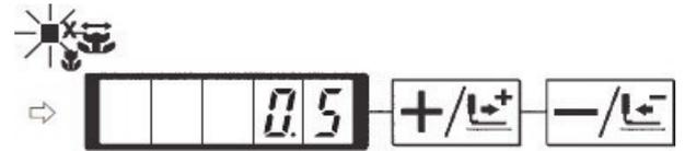
8. Press to activate Y scale rate , which is displayed at 0.0. The stroke in Y direction can be changed in step at 0.1mm. Use & to set that value at
